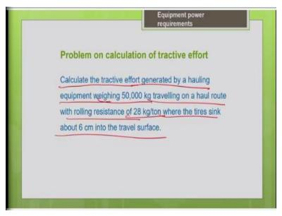
Now, for better understanding, let us work out a problem on calculation of the tractive effort. So, calculate the tractive effort generated by a hauling equipment, it is gross weight is given as 50,000 kg, it is traveling on a haul route. It is rolling resistance is given to you directly you can take it from the literature for that particular haul route; it is given as 28 kg per ton. And another important thing to be noted is your tire is sinking about 6 centimeters into the travel surface.
