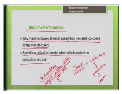
So, there are some more important terms you need to learn with respect to the machine performance. Basically, speed is a very important parameter used to quantify the machine performance. Most of the contractors are interested in the speed of the particular equipment. Because speed will affect your cycle time of the machine that is going to affect your production of the machine, that is going to in turn affect the cost associated with the machine.
