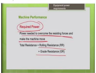
So, what is this required power? So, generally, what is the power needed by the machine to overcome the resisting forces in the project site and keep the machine moving, that is what is a required power. So, you know that every project site is unique, the underfoot conditions of the project site differs from site to site. So, the equipment which are going to use in a particular construction project site has to overcome all the resisting forces in the particular project site.
