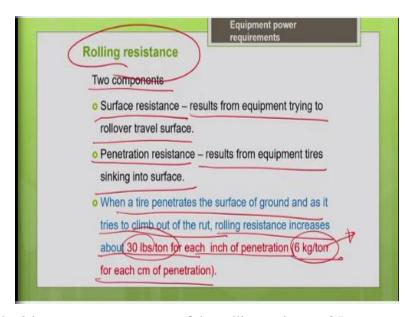
So, what are all the 2 important components of the rolling resistance? Let us see, one is the surface resistance other one is your penetration resistance. So, you can break this rolling resistance into 2 components, one is at the surface. So, the resistance which is encountered at the surface when the; wheel is moving over or rolling over the surface that is surface resistance.
