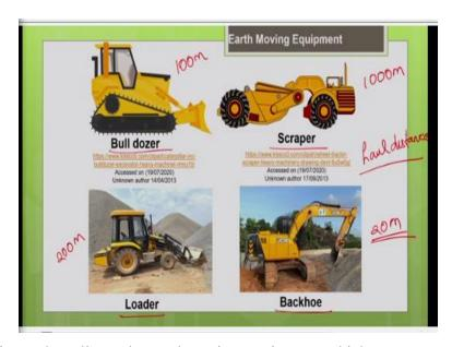
So, let us look into what all are the earthmoving equipment which are commonly used for the earthmoving operations. So, you can see this bulldozer, this is a scraper, this is the loader, front end loader and this is a backhoe, we call this an excavator. So, basically which equipment we need to select depends upon your project requirements. We have discussed about the factors influencing the selection of the equipment in the lecture 1, hope you remember.
