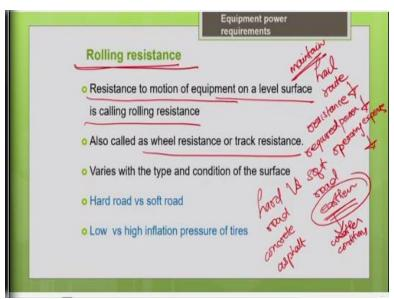
The first thing we will discuss about the rolling resistance. Rolling resistance is nothing but what is the resistance offered by the hauled route to the wheel which is rolling over the particular surface. So, what is the resistance offered by the hauled route to the wheel which is rolling over the particular surface, so that is what is your rolling resistance. So, resistance to the motion of equipment on a level surface is called as rolling resistance.
