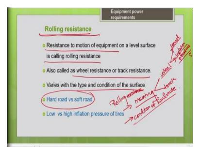
As I told you, it varies a lot with the type and the condition of the surface. And also, it depends upon the mountin, it depends upon the condition of your surface, condition of your hauled route. So, mounting in the sense, it can be either a wheel mounted or it can be a track mounted. If it is wheel mounted, even your dimension of your tyre, the tread dimension of your tyre and the inflation pressure of your tyre, all these things are going to affect your rolling resistance.
